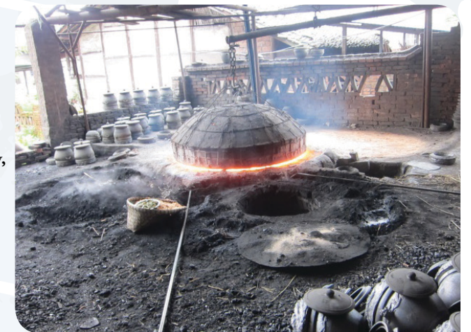
Removable ceramic kiln lid with pots being fired
